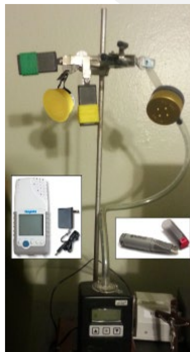
Figure 2-3. A typical indoor sampling setup used in the STOVE study contained monitors to measure the following pollutants (from left to right): formaldehyde (rectangular green), nicotine (circular yellow), NO_2 (rectangular yellow), and PM_{2.5} (circular gold). The device labeled “Telaire” (lower left) was used to measure CO_2 , temperature, and relative humidity. The gray device with the red cap (lower right) was used to measure CO.
